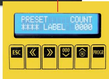
Automatic Label Counter Series allows to count the labels on a roll, to rewind and unwind the labels on one machine, to rewind the labels onto different core sizes, to rewind small rolls of labels from a larger one and also to rewind small rolls with a preset number of labels from a larger roll.
