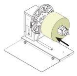
**STEP 4**Load the roll onto the core holder.
