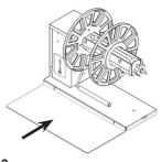
**STEP 2**Set the included printer plate beside the unwinder's plate.
