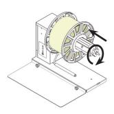
**STEP 5** Insert the outer disc onto the core and screw the knob.
