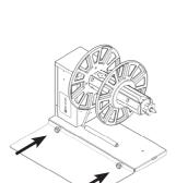
**STEP 3**Use the two knobs to fasten the printer plate to the unwinder's plate.
