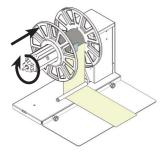
**STEP 5** Insert the outer disc onto the core and screw the knob.
