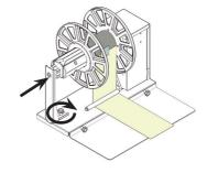
**STEP 6**Install the support and fasten it to the base through the knob.
