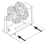
**STEP 3**Use the two knobs to fasten the printer plate to the rewinder's base.
