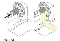
Load the empty cardboard core, let pass the printed media underneath the tension arm and stick it on the core.
