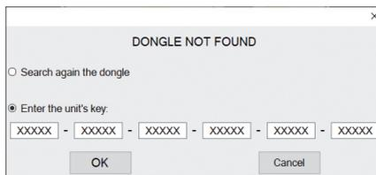
**Cause:** This occurs after opening the software while the dongle (the red key) was not plugged into the internal hub. This can also take place when the USB cable from the unit was not plugged to the pc or when you’re first installing the software.
