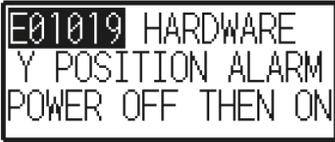
**Problem:** The plotter displays an error “E01019 Hardware Y Position Alarm Power off then on”.
