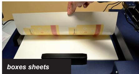
**WARNING** "When loading, sheets must not be bent over or damaged".
